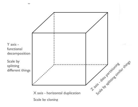
The two readily known scaling dimensions are X-axis scaling, which consists of running multiple identical copies of the application behind a load balancer, and Z-axis scaling (or data partitioning), where an attribute of the request (for example, the primary key of a row or identity of a customer) is used to route the request to a particular server.
