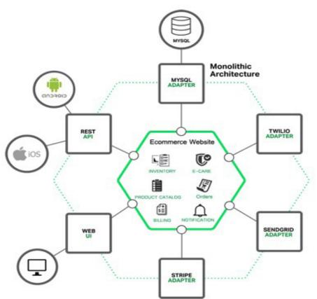
The system may be architected with modularity in mind, but code is stored in a single code base When it comes to packaging and deploying, you create one or a few huge executables. This deployment of large files exists even with minor changes. Although there are benefits, the downfalls have led to this newer microservice architecture.
